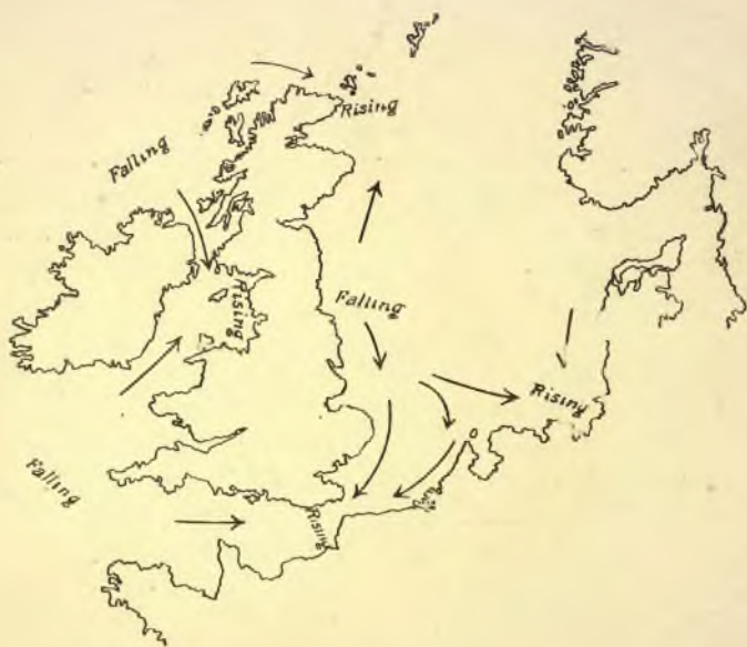
FIG. 24.—The approximate set of the tidal currents, when the water is rising at Liverpool.
