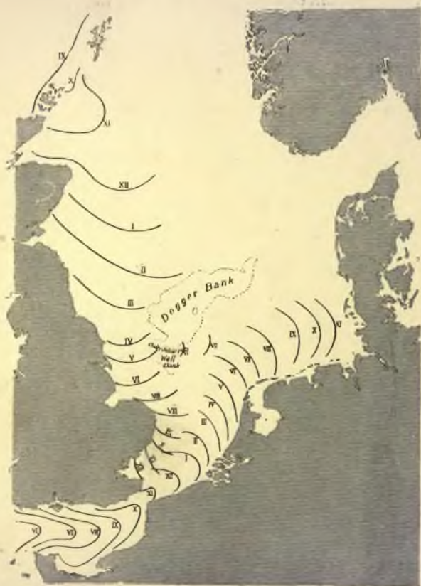
FIG. 23.—The hours of high water in the Narrow Seas, when noon is the hour of high water at Liverpool.
