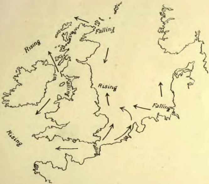
FIG. 25.—The approximate set of the tidal currents, when the water is falling at Liverpool.
